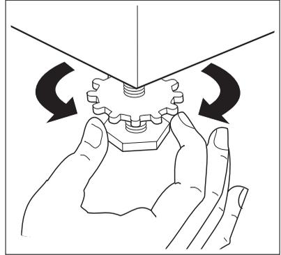
After having levelled the appliance, tighten the lock nuts.
